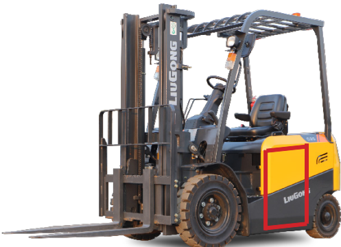
Battery sink down
